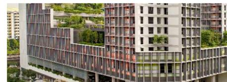
**Image 5: Careful glass selection for external façade and extensive sun-shading elements to reduce heat gain into the building.**
